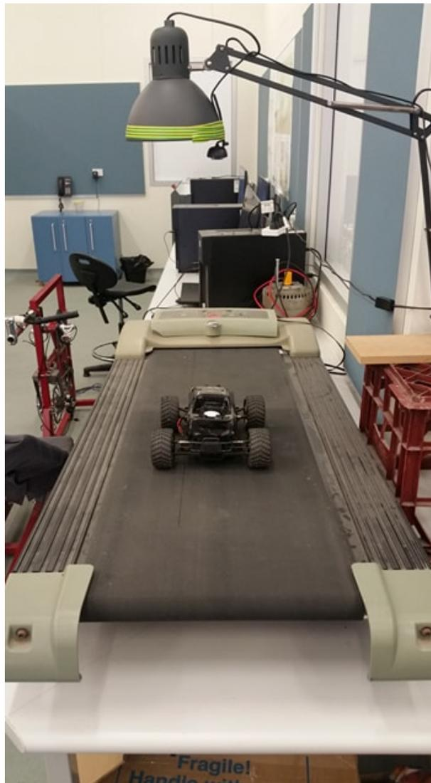
**Figure 3.3:** The moving ground, vehicle model, camera mount and camera apparatus.
